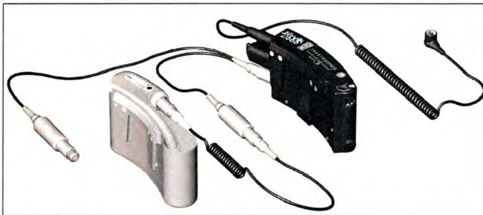
External Equipment for Jarvik 2000® VAS, Post-Auricular Cable.
